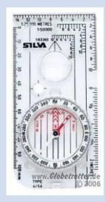
A compass can be used to work out which direction to travel in. The compass uses the earths natural magnetic fields which moves the needle and allows the user to find North. Compass can be used in orienteering to find locations on a map.
